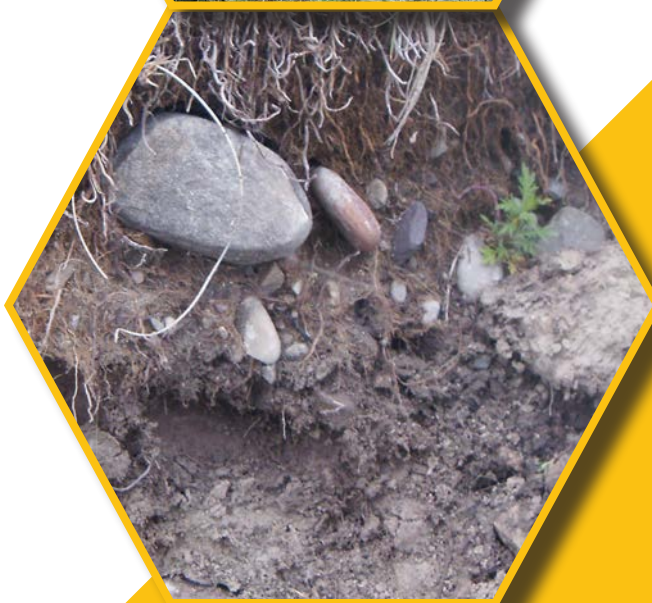
Pinched out gravel shows how close to the surface the gravel zones are.
